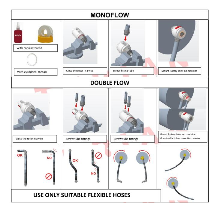
Rotary Joints are precision devices that need to be handled with care for proper operation. For a correct installation please proceed as follow:
