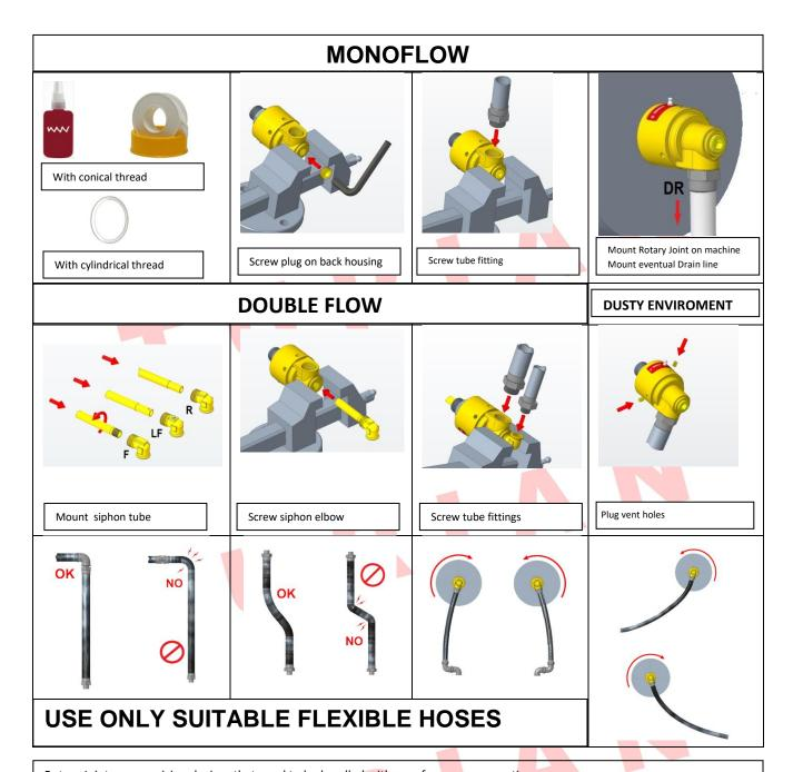
Rotary Joints are precision devices that need to be handled with care for proper operation.
